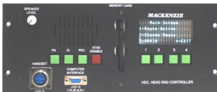
The Head End Controller(HEC) is the operator interface to Mackenzie's transit communication system. The HEC gives the operator a single user-friendly interface for controlling the various communications systems of a transit vehicle.
